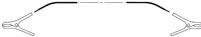
CRIMP ELECTRICAL CLIP TO ELECTRICAL WIRE AND SOLDER
